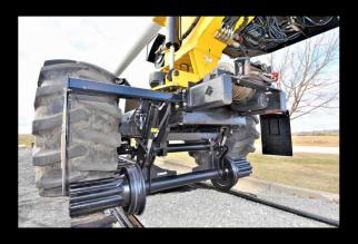
Mitchell Friction Drive for Rubber Tired Jarraff Tree Line Trimmer allows the machine to self-propel on the railorad track to work on rail or work on the ground with the friction Drive Hi-Rail Gear retracted. The configurations allows the blade to remain on the machine for working on the ground. When working on the rail the blade can be lowered to sit on the rail to add additional stability.
